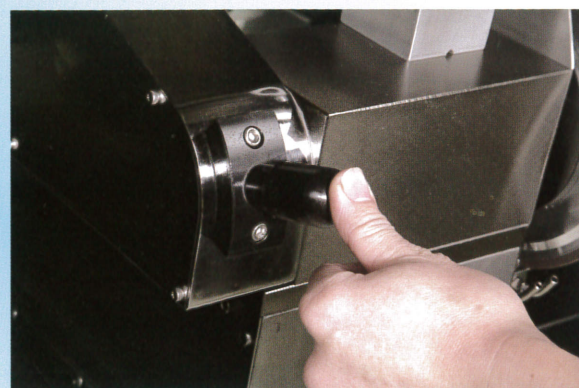
Locking Device for Grinding Wheel Dismantling 砥石取り外し用固定装置
