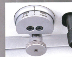
Grinding wheel tilting adjustment 砥石上下移動量
