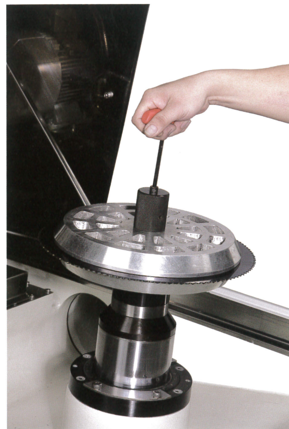
Patented Sawblade Locking Device Design 鋸固定装置
